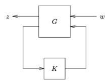
Fig. 1. Closed-loop system.
